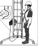
Ascend ladder to desired position. Use work positioning hook to attach
