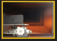
★ Light Tunnel: Photometric Validations to SAE standard for LED, Fluorescent, Strobe, Halogen and Incandescent
