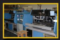
Thru-hole automation insertion equipment
