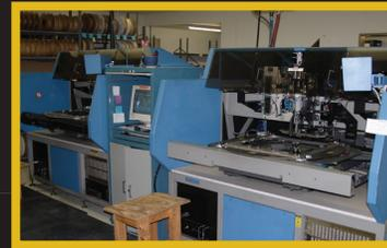
★ Thru-hole automation insertion equipment
