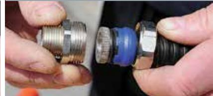
Bring the body to mate with the back nut. Metal fittings should be tightened with grips or spanner to ensure security and IP rating.
