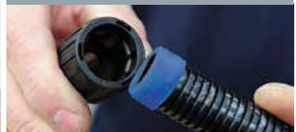
The FPAX fitting features a conduit seal to provide the ultimate IP rating up to IP69K. This simply fits onto the end of the conduit before the fitting is connected to the conduit. To aid assembly moisten this seal. An FPA fitting cannot be uprated to IP69K with the addition of a seal. Pull back slightly to ensure the locking teeth mechanism has engaged with the corrugations.
