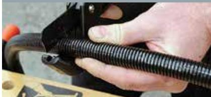
Non-metallic conduits and FLP up to 34mm can be easily cut with Flexicon Conduit Cutters, part no. CC01. Use CC02 for sizes up to 67mm. Drop the blade into a corrugation and squeeze and twist until conduit is cut 50% through. Cut the remaining 50% without twisting to achieve a square cut.
