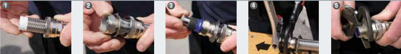
Our type-C braided fittings consist of an outer compression nut, an inner compression nut, an elastomeric seal, an insert and a body. Firstly place the outer compression nut on the conduit as per 1. Remove the tape securing the braid and pull back to allow the inner compression nut to be fitted as per 2. Next, fit the elastomeric seal (note the orientation) and screw the insert into the end of the conduit until this gives a secure fit as per 3.
