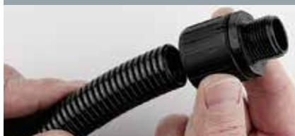
For Flexilok® and FPA fittings simply push the conduit into the end of the fitting with a slight twist until it will go no further. Pull back slightly to ensure the locking teeth mechanism has engaged with the corrugations.
