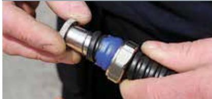
Firstly place the back nut on the conduit followed by the seal (note the orientation). Next, screw the insert into the end of the conduit until this gives a secure fit.
