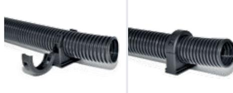
Ensure the hinged lid is open and insert the conduit from above. The clip size is shown on the clip for easy reference. The clip provides a secure fit whether the hinge is open or closed. The FCL clip includes an internal rib to help locate and retain corrugated conduits. The FCL-P clips do not have this rib and can therefore be used with plain or smooth outer conduits.
