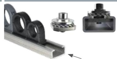
The **MRFAH** products can be inserted from the end of the rail. The **MFRAH** has a serrated washer to offer anti-vibration performance. It clamps on the top rail to secure the fittings.
