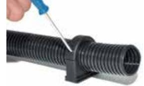
To remove the conduit insert a small screwdriver where it states OPEN. Push down and lever to release. The hinge should then be free to open.
