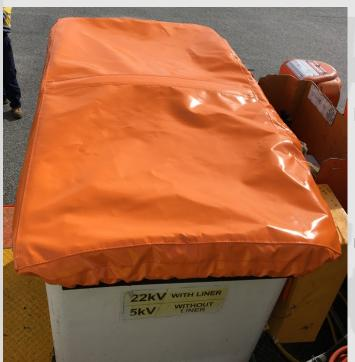
Custom made EWP Bucket covers to protect your bucket this Winter! Has integrated Aluminium Flat bar for runoff and sewn in Bungy cord.
