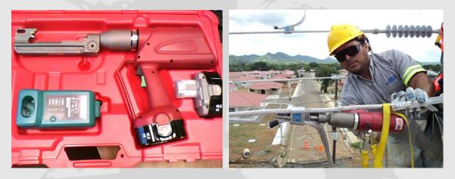
We are pleased to announce the introduction of our new line of battery actuated WEJTAP connector installation tool. These self contained battery powered WEJTAP hydraulic tools use a combined proven platform of WEJTAP tool heads and 18volt Ni-MH battery hydraulic tools to offer a reliable WEJTAP Tool that does not require explosive booster cartridges!
