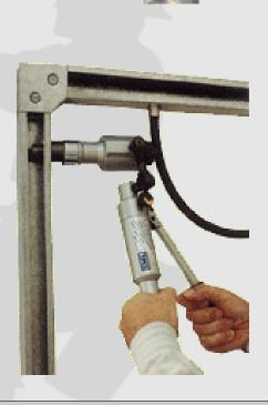
Max round Hole 60 mm Max square Hole 46 x46 mm
