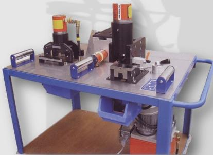
A Complete work-station with electro-hydraulic pump. (220 volt, single phase), machine selector-switch and 3 separate machines for cutting, punching and bending. The machines are carefully positioned to give free access of the copper bar to each machine.
