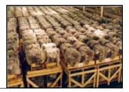
ZERUST® ICT®510-C FERROUS YELLOW FILM USED TO LINE A SHIPPING CONTAINER AND WOOD PARTITIONS FOR THE PROTECTION OF GEARS DURING SHIPMENT FROM WESTERN EUROPE TO ASIA.
