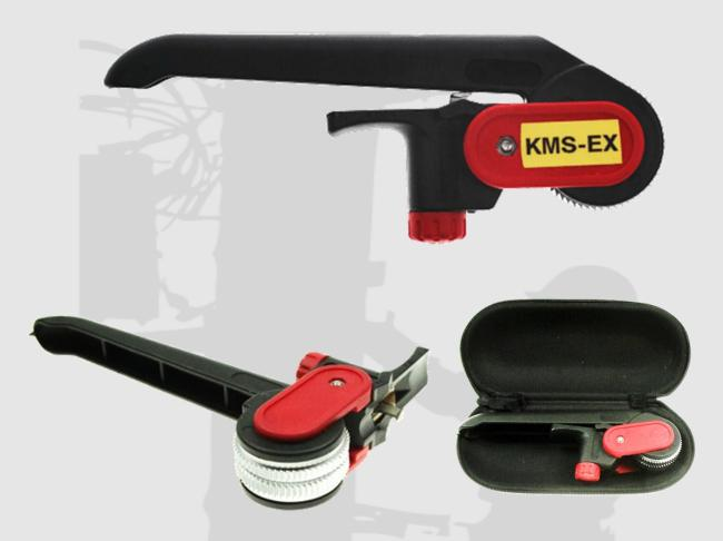
Designed for the removal of the outer XLPE sheath quickly and easily on all large size cables with a ratchet up and down action the stripper moves along the cable cutting the sheath as it goes.
