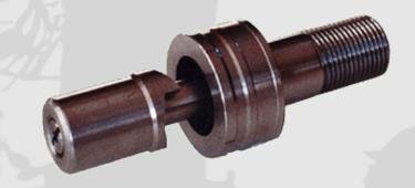
As a result of the splitting action of the Bulldog punch, the pilot hole needs only be slightly larger then the tie bolt (0.2mm clearance). This ensures that a row of holes will be perfectly inline.
