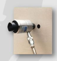
Max round Hole Diameter 120mm Max square Hole 92x92 mm Max steel Thickness 3 mm Hose Length 800m Total Weight 9.4 Kg Max Pressure 500 bar
